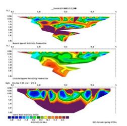
Measuring the resistivity of a soil provides an indication of its moisture content, and although this is a well researched topic, work on fine grained London clay is relatively new and very relevant to our understanding of how moisture moves in relation to root extraction.
